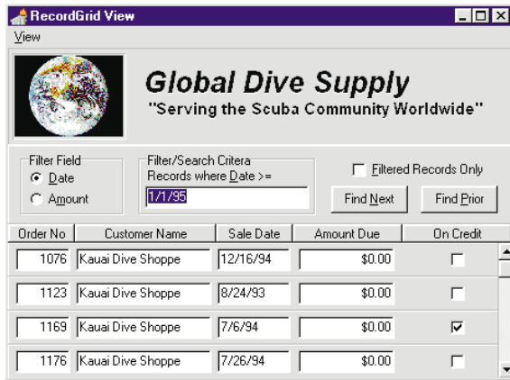
Figure 8: The new DBCtrlGrid component gives you greater flexibility in presenting multiple records of data.
